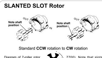
Diagram of 7-roller rotor with special slanted, wide roller slots (Series
